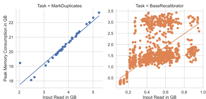
Fig. 2: Memory consumption in relation to the input read of the physical task instances of two different task types, with a linear regression applied to these data points.
